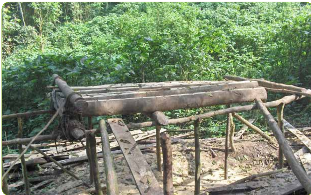
Figure 5 A fresh pitsawing platform recorded on 16th December 2015
